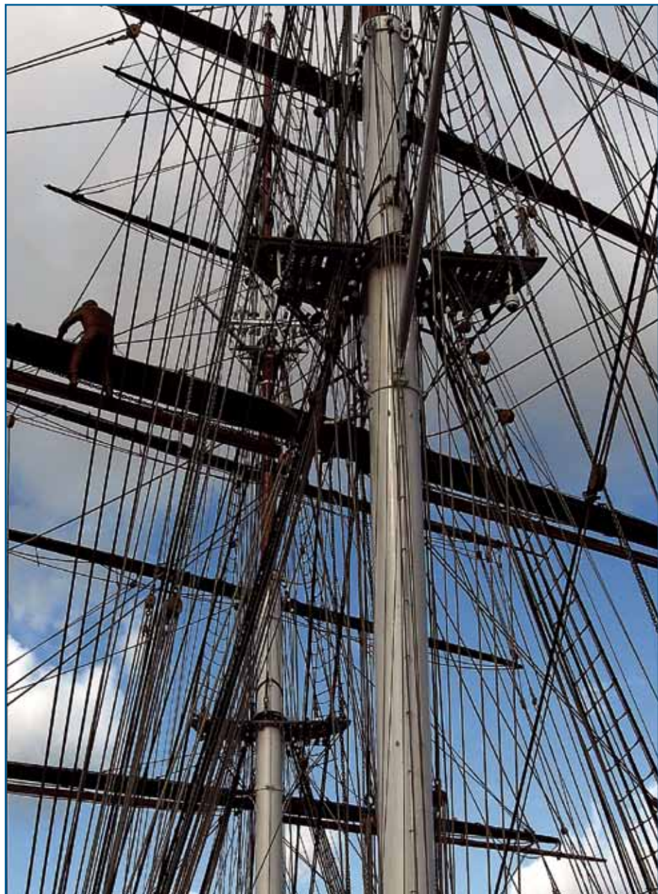
The rig was designed for the tea route with "skysails" above the royals and stands 152 feet above the deck. In light winds, the square sails were supplemented by extending "stunsail" booms carried under the yards. Lifesize figures in the rigging give a sense of scale
