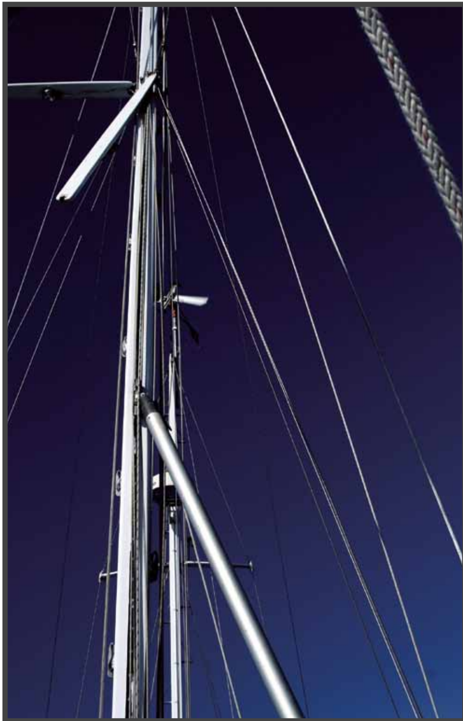
The broken port spreader hangs from the shroud before it finally detached completely from the mast.
