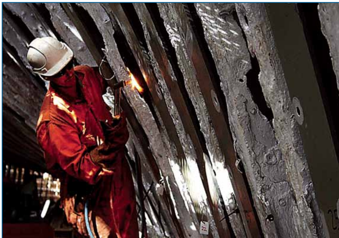
Photo above - This view of the bow from below the waterline shows the fine entrance and hull shape that made the clipper the fastest sailing cargo ship ever built, and a symbol of progress in the 1800s. Photo below - Restoration of the corroded iron hull frames was not greatly affected by the fire, but required intensive chemical treatments over many years.
