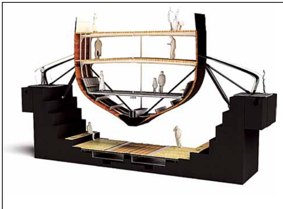
This artist's impression shows how the ship is suspended without the hull deforming. It took several days to jack the ship and connect the props.
